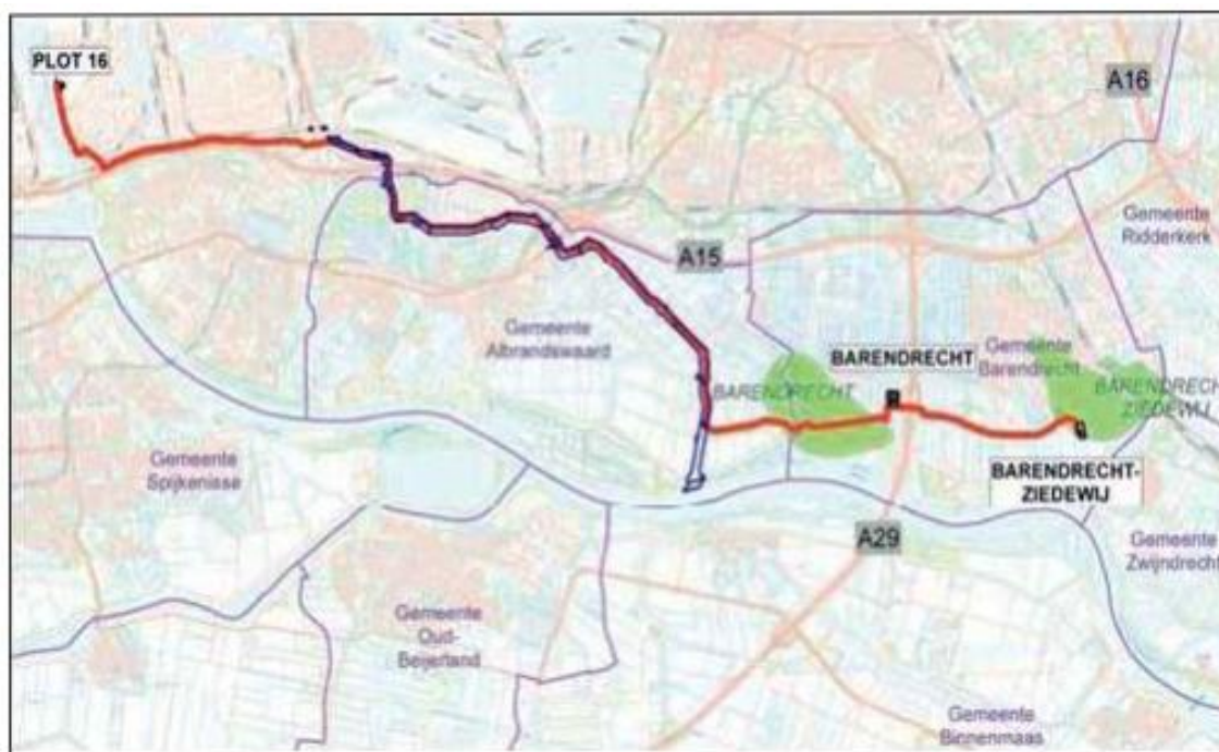
Figure 5.2 Location of the planned CO 2 pipeline and gasfield in Barendrecht (Source: Shell CO 2 Storage, 2008)
